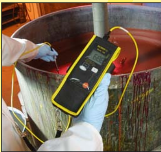
Temperature measurement in hazardous areas
