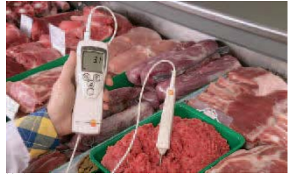
Monitors temperature in refrigerated counter
