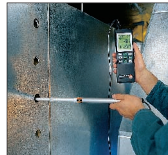
Volume flow measurement using timed and multi-point mean calculation
