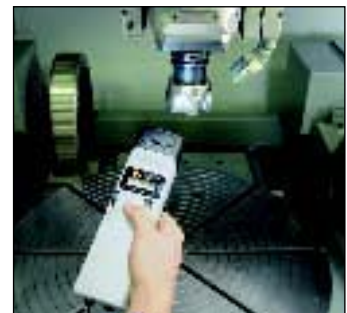
The creation of a stationary picture enables the inspection and qualitative assessment of high frequency moving parts
