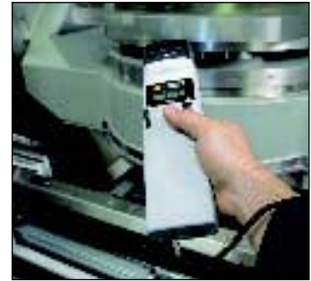
Measures the speed e.g. in rapid stroke machines
