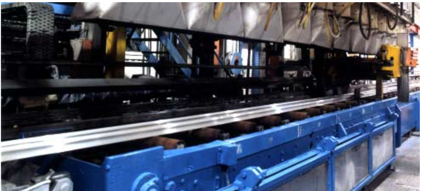
Typical air quenching system on an aluminium extrusion line
